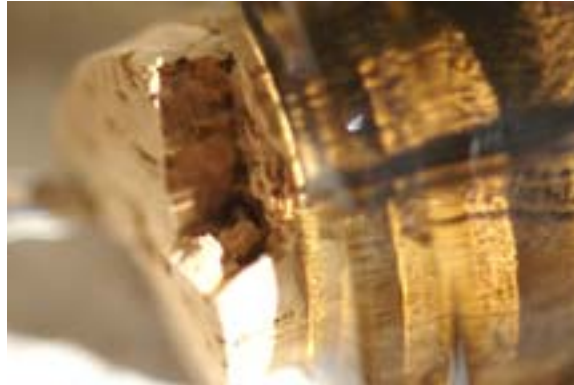
Figure #4: Close up of the top of the bottle near the second fracture. This shows the damage to the cork when the corkscrew was first inserted.
