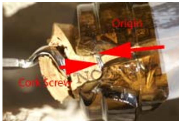
Figure #5: Photograph of the re-assembled neck. This shows the second fracture on one side of the neck. This failure was caused by the side of the corkscrew being driven into the inner wall of the bottle. The two halves of the fracture are parted because the cork has expanded since it is no longer squeezed in the neck.
