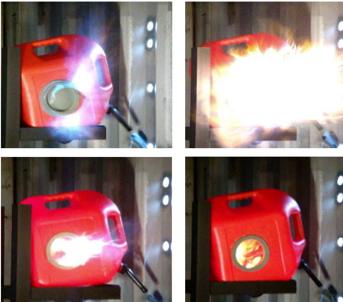
Figure 6. Gasoline cans tested w/o flame arresters from 4 separate tests with gasoline in the explosive range.
