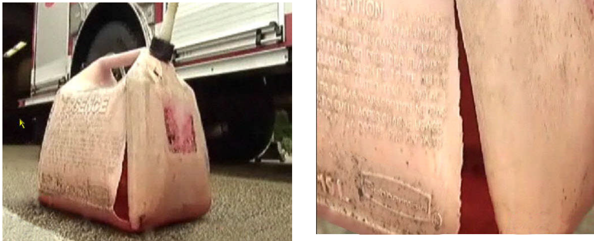
Figure 1. Subject gasoline can showing clear signs of explosion and rupture.
